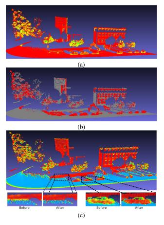
Fig. 2. Robust neighborhood filtering. Values of  $\sigma_p$  (a) and values of  $v_{nz}$  (c) are visualized in color with redder being smaller and bluer being larger. In (c), we also show two zoomed-in details of intersection areas before and after robust neighborhood filtering. All points that pass both point-ness thresholding and dominant plane criteria are highlighted in red in (b).
