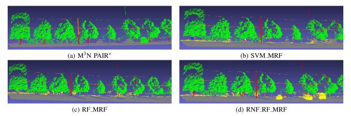
Fig. 3. Comparison of six-category classification results on a sample scene using *Oak05* for training. Color scheme: green-vegetation, orange-wire, red-pole/trunk, gray-ground, blue-facade, yellow-vehicle
