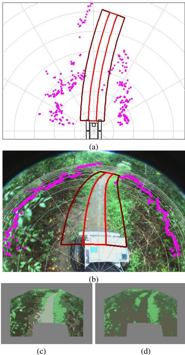
Fig. 3. (a) Robot with candidate trail region and neighboring regions, ladar hits (grid circles are at 1 m intervals); (b) Candidate trail region, ladar projected to camera; (c) **LAB** space  $k$ -means labels (colored with mean RGB of each cluster; gray frame is mask); (d) **AB** space  $k$ -means labels
