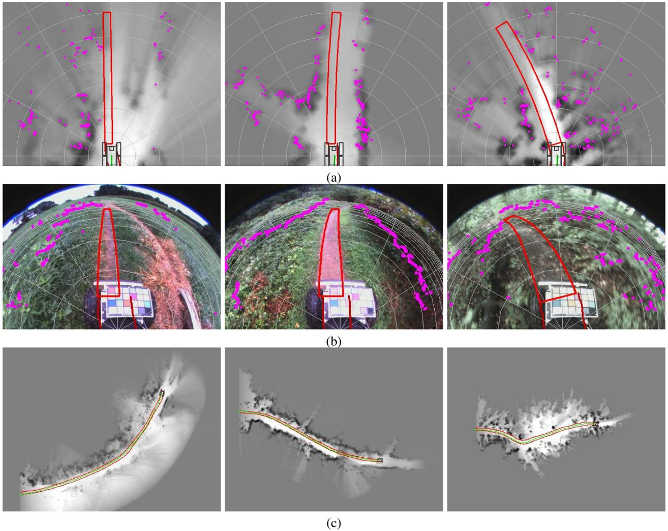
Fig. 5. (a) Local occupancy grids at current robot location created using visual odometry information during runs along *field*, *mixed*, and *forest* (from left to right); (b) Camera view at current location with current tracked trail state overlaid; (c) Partial global maps with trail and position histories overlaid
