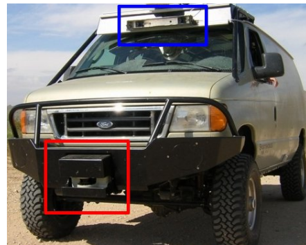
Fig. 1. Vehicle used to capture data for this paper. The ladar is mounted on the bumper (indicated by the red box) and the camera is one of the stereo pair over the windshield (the blue box).
